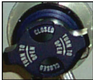
Reservoir Depressurization Valve (installed on each Hydraulic service panel)
